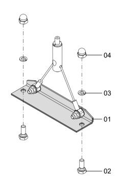
OM100 suspension bracket with Y-Steel rope
