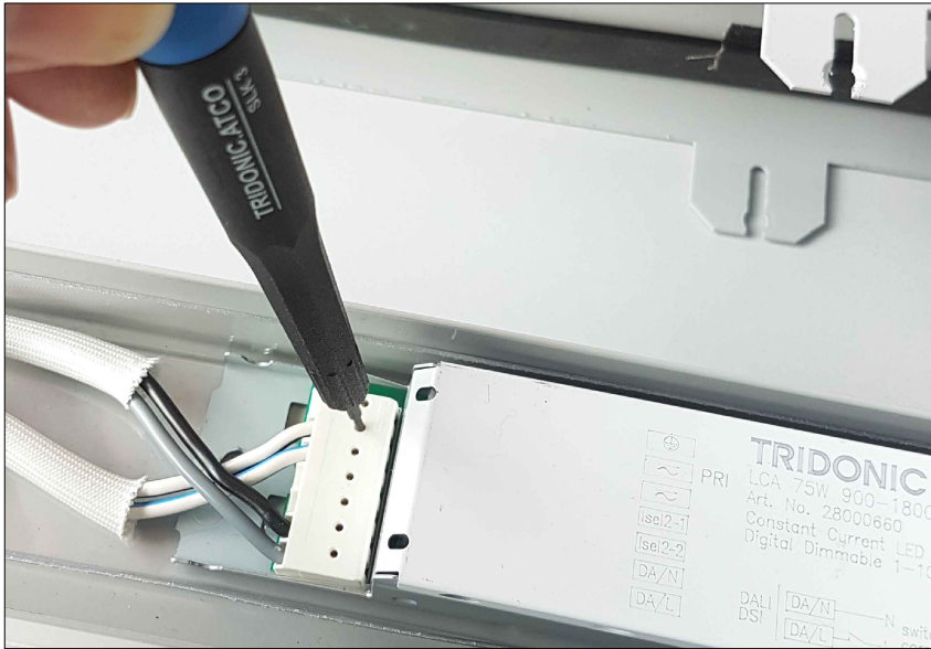
6) loosen the wires on the primary side with a suitable tool
