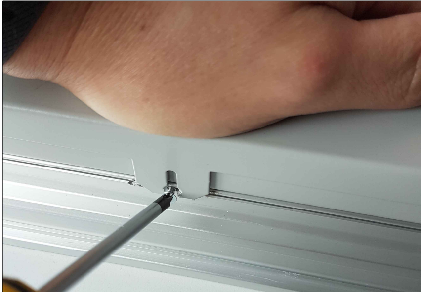
14) place the cover with pressure and screw it from the center
