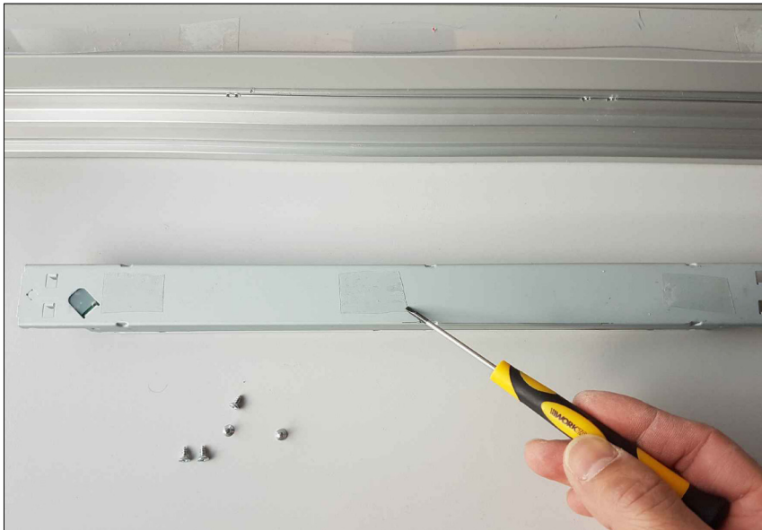
10) equip new driver unit with double-sided adhesive tape
