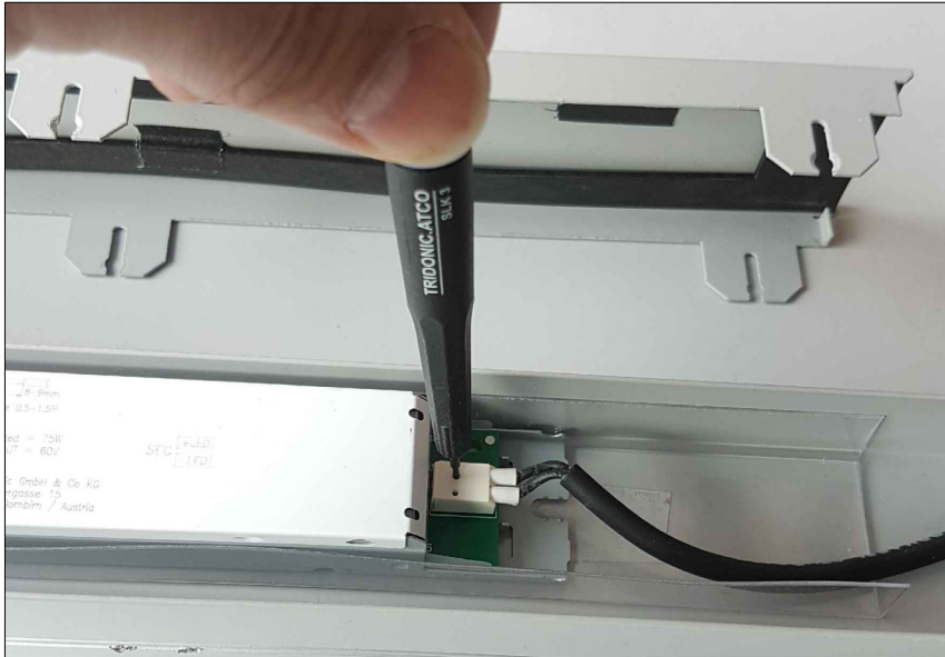
7) loosen the wires on the secondary side with a suitable tool
