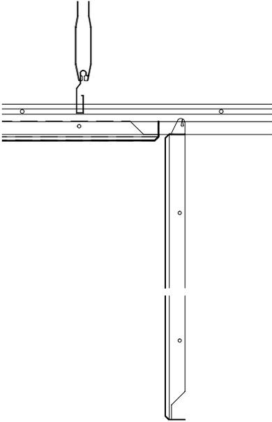
6. To remove the metal tile from the clip-in carrier, the carrier must be spread open with a screwdriver.
