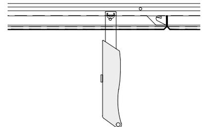
3. Pull the metal tile down until no more resistance is felt.
